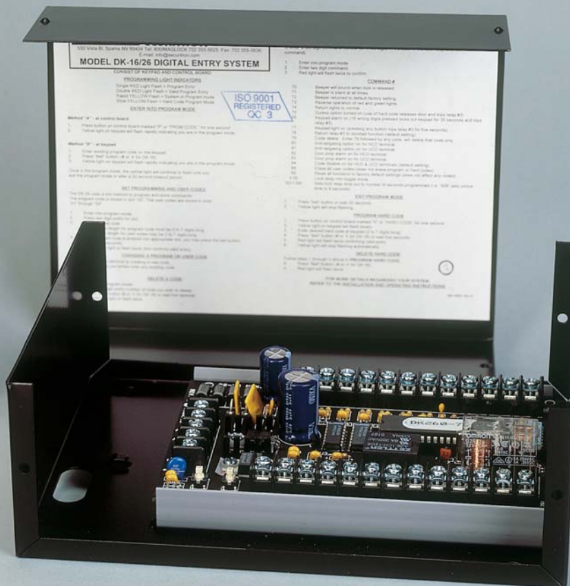
REMOTE CPU IN STURDY STEEL CABINET
