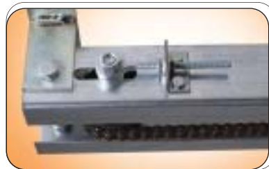
chain tensioner allows for quick and easy chain adjustment
